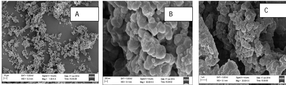
Figure 5: SEM images of the biosynthesized ZnO nanoparticles.
