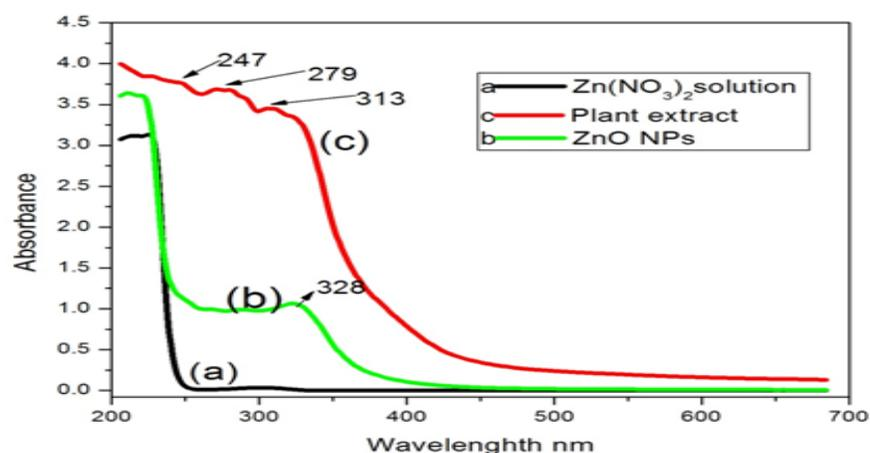
Figure 1: Comparison UV-Vis spectra for Zinc nitrate solution (a), ZnO NPs (b) and plant extract (c).
