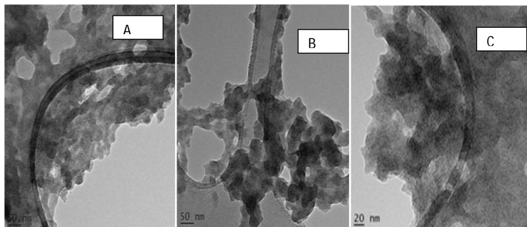
Figure 3: TEM images of biosynthesized ZnO nanoparticles (A-C).
