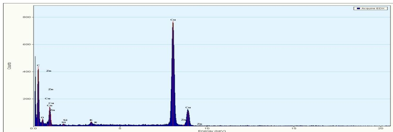
Figure 4: EDX elemental analysis of ZnO nanoparticles.
