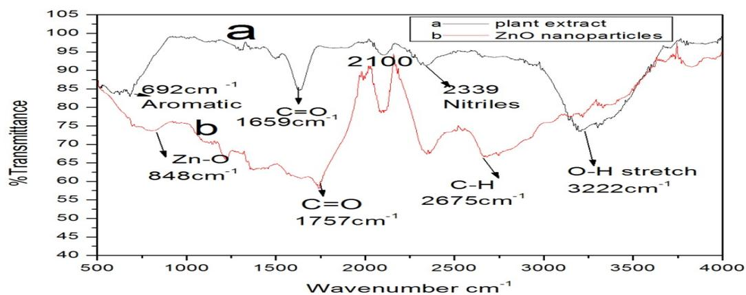
Figure 6: ATR FT-IR spectra of (a) plant extract, (b) ZnO nanoparticle.
