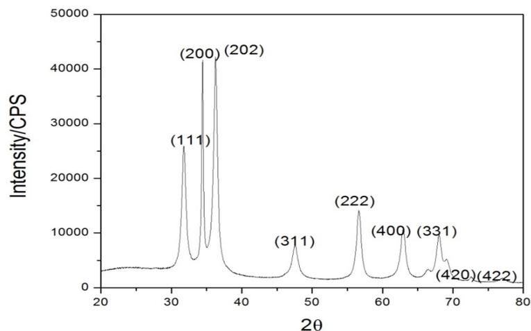
Figure 2: XRD pattern for the biosynthesized Zinc Oxide nanoparticles.
